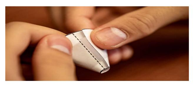
The system uses a regular piece of paper cut and folded into a funnel to guide sound waves in and out of the ear canal. Dennis Wise/University of Washington
